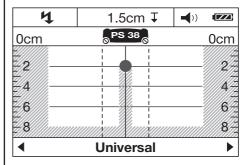
A live metallic object, e.g. an electric cable, is within the sensor area. It lies at a depth of approx. 1.5 cm (0.6 in). The tool emits a warning signal tone for "live cables" as soon as the electric cable is detected by the sensor.
