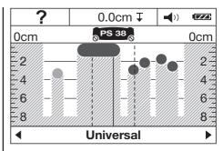
Switch to "Hollow brick" mode. Most of the cavities will then no longer be shown in the display.
