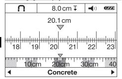
The display mode can be changed in all scanning modes. This function changes only the display mode, not the scanning mode.
